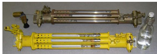
batometre de tip Nansen (foto: slideplayer.com )
